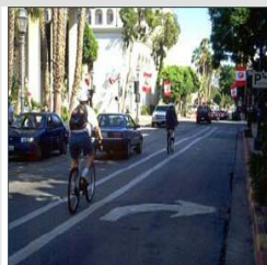
Turn pockets: Narrow lane at intersections where bicycles turning against the flow of traffic can wait safely and be highly visible.
